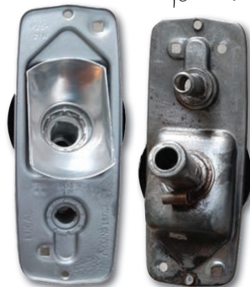
The old Lucas light units were cleaned and painted.
