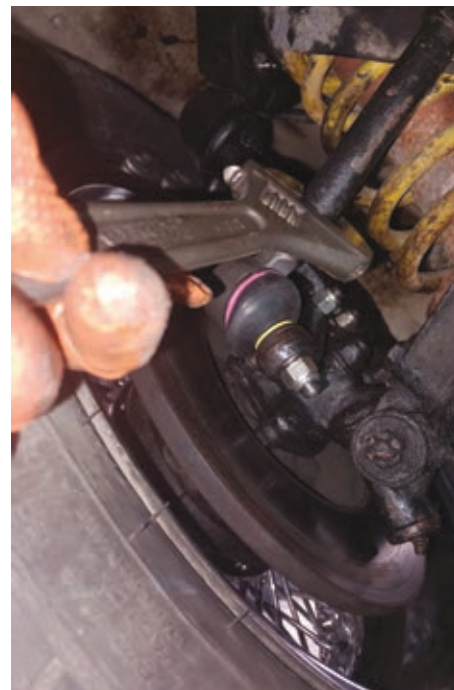
7. It took several tweaks to get the toe-in/toe-out right.
