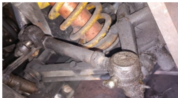
3. The tie rod control bearings were well worn...
