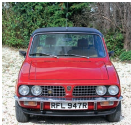
The Dolomite's 53.2in track was 86.2% of its overall width, a wide stance clear to see in this picture.
