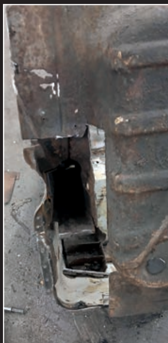
The front tub has had new body mount/A-post sections from Chic Doig, and repairs to the windscreen frame/drip channels.
