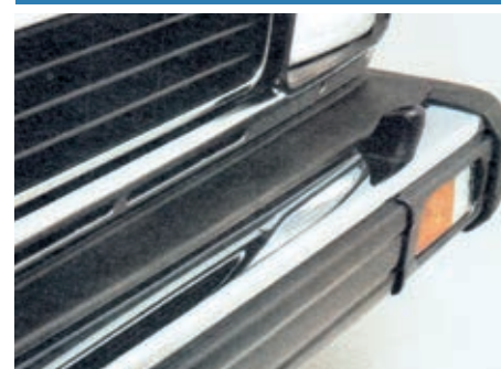
Only the Acclaim CD featured headlight pressure washers (above) and bright bumpers (below).
