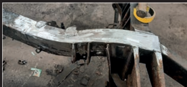
The chassis needed the usual repairs on the main rails around the diff and at the base of the boot outriggers.
