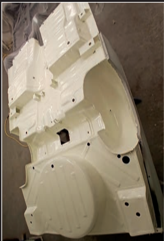
Most of the body panels are now in epoxy, with underneath of the body tubs stonechipped and painted in Triumph White 19.
