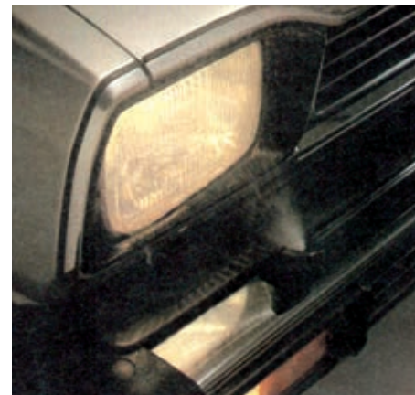
Only the Acclaim CD featured headlight pressure washers (above) and bright bumpers (below).
