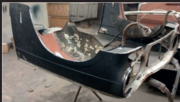
The bonnet assembly has had new wings, new inner arches (outer) and D-Plates.
