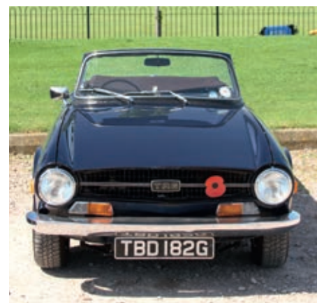
...while the older TR6 had a narrower track at 50.2in but a higher percentage of overall width at 86.6%.
