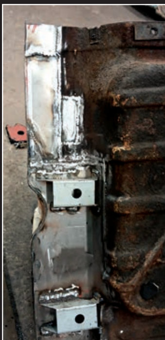
The front tub has had new body mount/A-post sections from Chic Doig, and repairs to the windscreen frame/drip channels.
