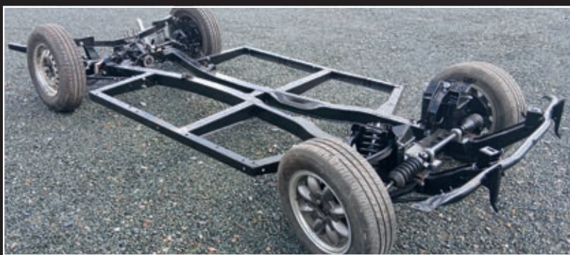
Chassis painted black and rolling, minus the rear spring which has been sent off for a refurb.
