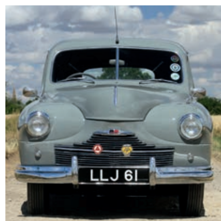
...while the Standard Vanguard Phase 1's modest 51in track was just 73.9% of its overall width.
