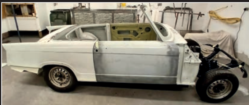
Body tubs back on the chassis, doors on and the tricky part of body alignment is about to begin.
